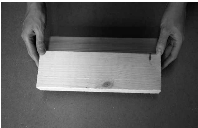
Glue (wood glue) the wooden pieces (those that are 29 cm) on top of each other. Half of the boards should be attached to each other.
