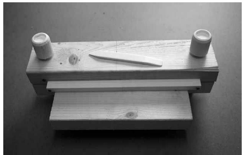
Then fix the cutting device onto the board with the screws. To increase stability, you can also glue the cutting device with contact adhesive before you screw it on (recommended).
